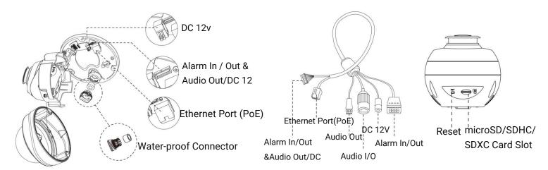
The cable is connected with the interface board by default.
