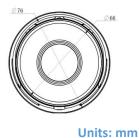
A01 V3 Pole Mount Weight: 625g Dimensions: 140\*136\*46mm
