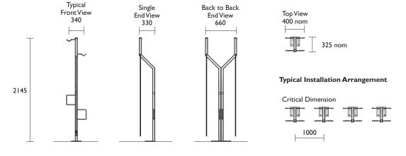
$\label{eq:material_specifications} \begin{tabular}{ll} Material Specifications (General) \\ 50 \times 50 \times 2.5 mm SHS / 12 Ø Rod / 6 mm MS Plate / Hot dipped galvanised PVC coated steel cable assembly \\ \end{tabular}$
