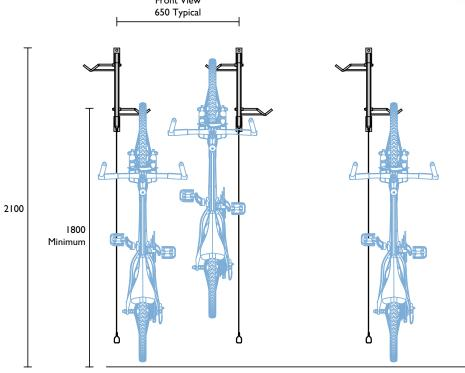
$\label{eq:material} \begin{array}{l} \textbf{Material Specifications (General)} \\ 30 \times 30 \times 1.6 \text{mm SHS} / \text{Hot dipped galvanised} \\ 100 \times 40 \times 6 \text{mm MS plate} / \text{Hot dipped galvanised} \\ \end{array}$
