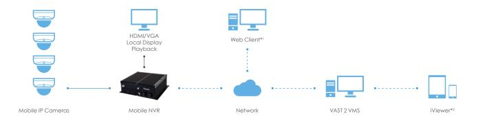
\*1: Available when Mobile NVR in static IP address.
